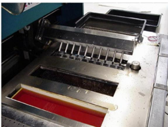
Fig. 1. Robotic hot solder dip system [4].
